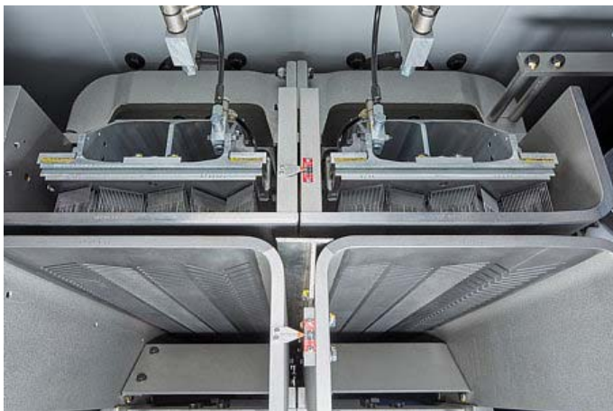
Needle arrangement "8000X" for a more even needlefelt surface
